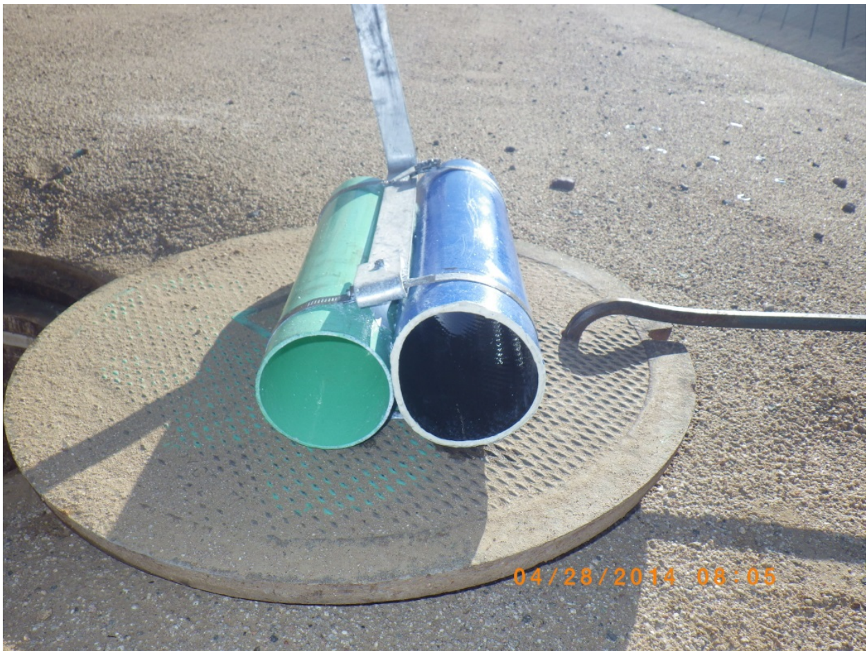
Figure 6: Test pipe apparatus used to monitor in-line scale accumulation.
