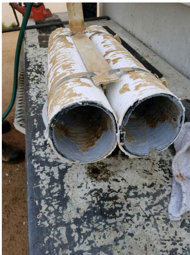
Figure 9: Test pipe verifying minimal scale accumulation within the discharge stream.
