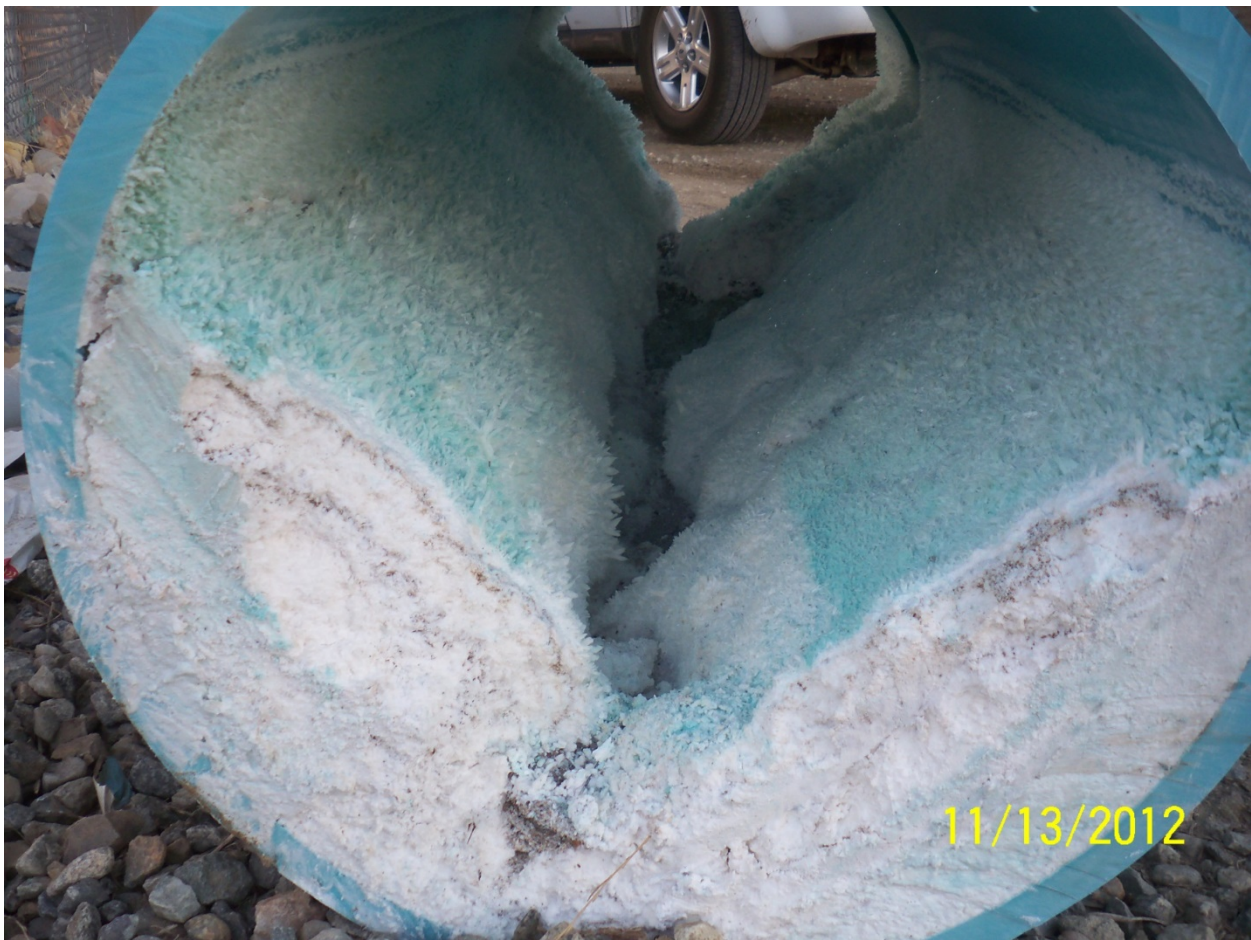
Figure 1: Section of scaled 16-inch diameter pipe, showing significant reduction in available flow capacity.
