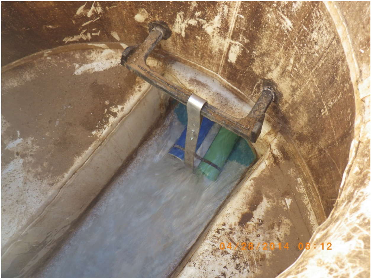
Figure 7: Test pipe apparatus submerged into pipeline flow to evaluate scaling.
