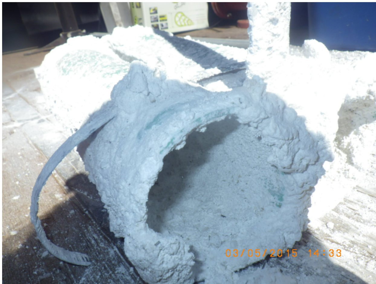
Figure 8: Test pipe verifying significant scale accumulation within the discharge stream in 2015.
