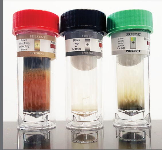
Day 5 BART showing a positive result for iron-related (left) and slime-forming (right) bacteria.
