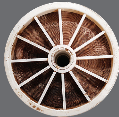
Pre-autopsied membrane element showing severe fouling.
